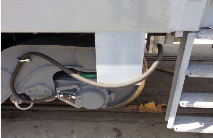
Fig. 13: Speed sensor installed on phonic wheel
