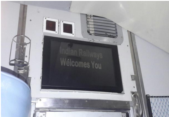
Fig.4: Passenger announcement/ passenger information system (PAPIS)
